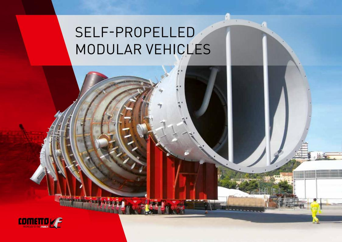
Cometto's MSPE electronic, self-propelled modular vehicles provide a complete transport system for industrial facilities, ro-ro operations and heavy load transports. The MSPE system includes different families with different characteristics, dimensions and bearing loads while maintaining central similarities that allow full interchangeability between different product lines.
